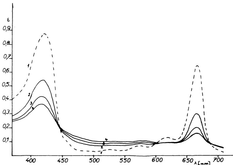
Fig. 4. Absorption spectrum of illuminated chlorophyll *a* in benzene ( $d = 10$  mm).
