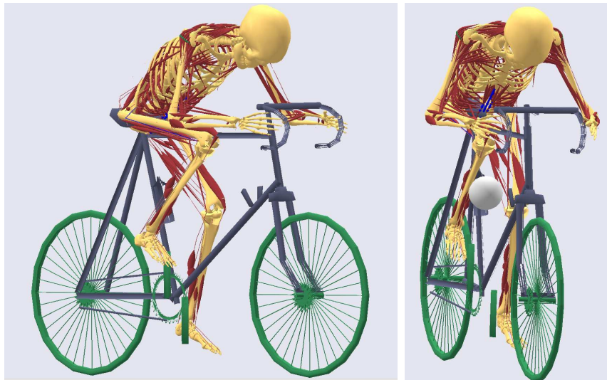
Fig. 1: A bicycling full-body model made in AnyBody by the AnyBody Research Group [2]. It comprises more than 400 muscles and all the major segments of the upper and lower extremities of the body as well as the spine. More than 150 of these use the string-contact model described in this paper. The bicycle is modeled by a single segment, the crank, whereas the rest is pure visualization.
